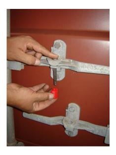
3. <u>Test Seal:</u> Pull firmly downwards on the plastic piece to confirm that the seal has been properly locked.
